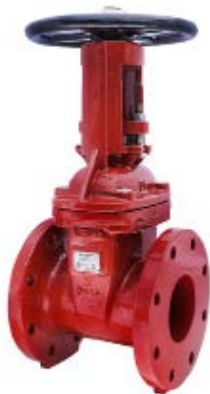
OS&Y Gate - FxF, GxG, FxG Ductile Iron 300/250/200 PSI | Sizes: 2½" - 24" AWWA C515 & C550, NSF-61 & 372
