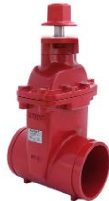
NRS Gate - GxG Ductile Iron 300 PSI | Sizes: 2½" - 12" AWWA C515 & C550, NSF-61 & 372
