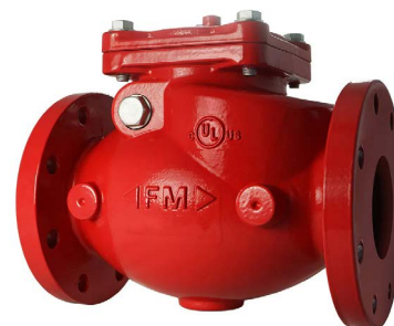
Swing Check - Flanged Ductile Iron 300 PSI | Sizes: 2" - 12" AWWA C508 & C550
