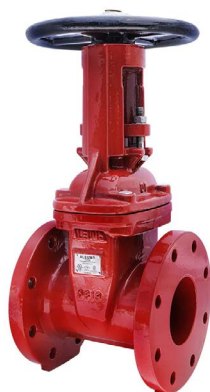
OS&Y Gate - FxF, GxG, FxG Ductile Iron 300/250/200 PSI | Sizes: 2½" - 24" AWWA C515 & C550, NSF-61 & 372
