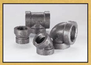
Ward Class 125 cast iron fittings are rugged, strong and make up tight. A chamfer is cut or cast in all openings, permitting easy engagement of pipe and preventing damage to the first thread in handling and threading.
