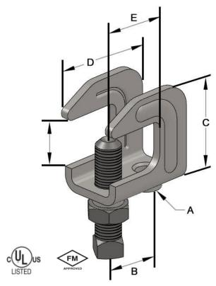
**Function:** Designed for attaching hanger rod to the top flange of a beam or bar joist, where the flange thickness does not exceed 3/4inch (19.05mm). The open U design permits rod adjustment.
